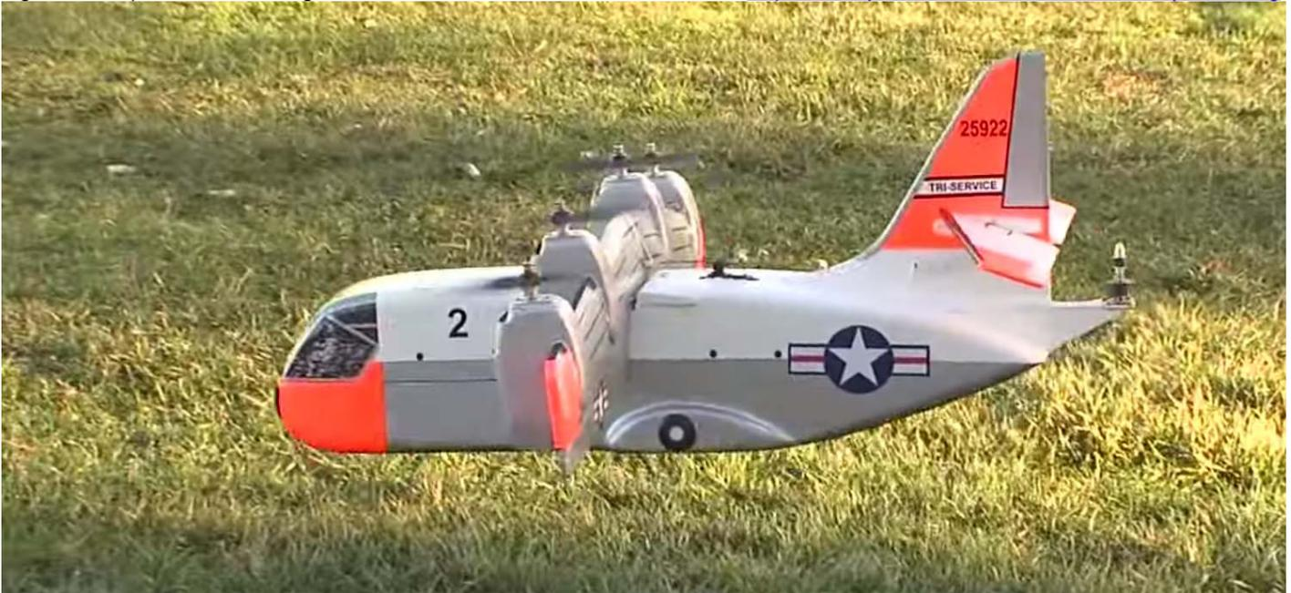
Here is a series showing the conversion from hover mode wing up through full transition to forward flight wing down.
