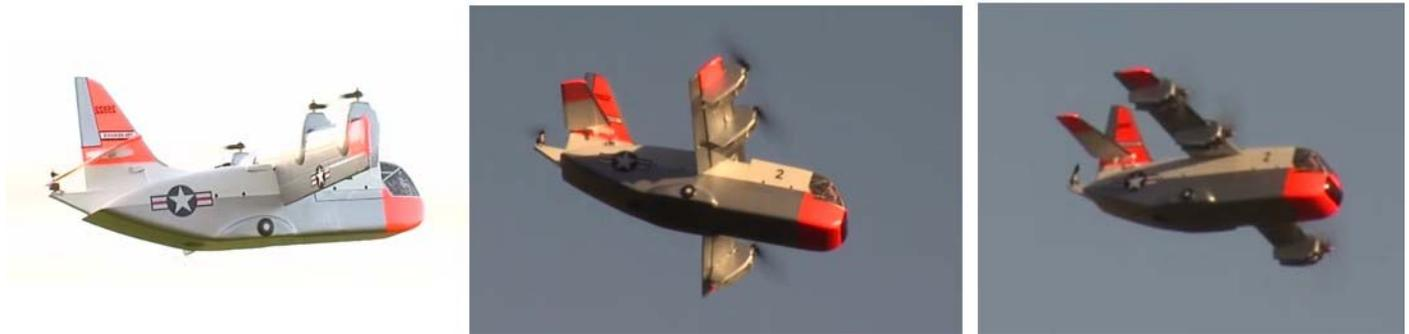
The model is a very simple scratch built foam design with conventional motors and controllers. Servos control wing tilt, ailerons/flaperons and horizontal tail incidence (elevator). Pitch control in hover and slow speed flight is via a small motor/propeller mounted vertically in the tail (just like the VZ-2). Yaw control in hover is via the flaperons in the wake of propellers and yaw control in forward flight is via differential propeller thrust, side to side.
