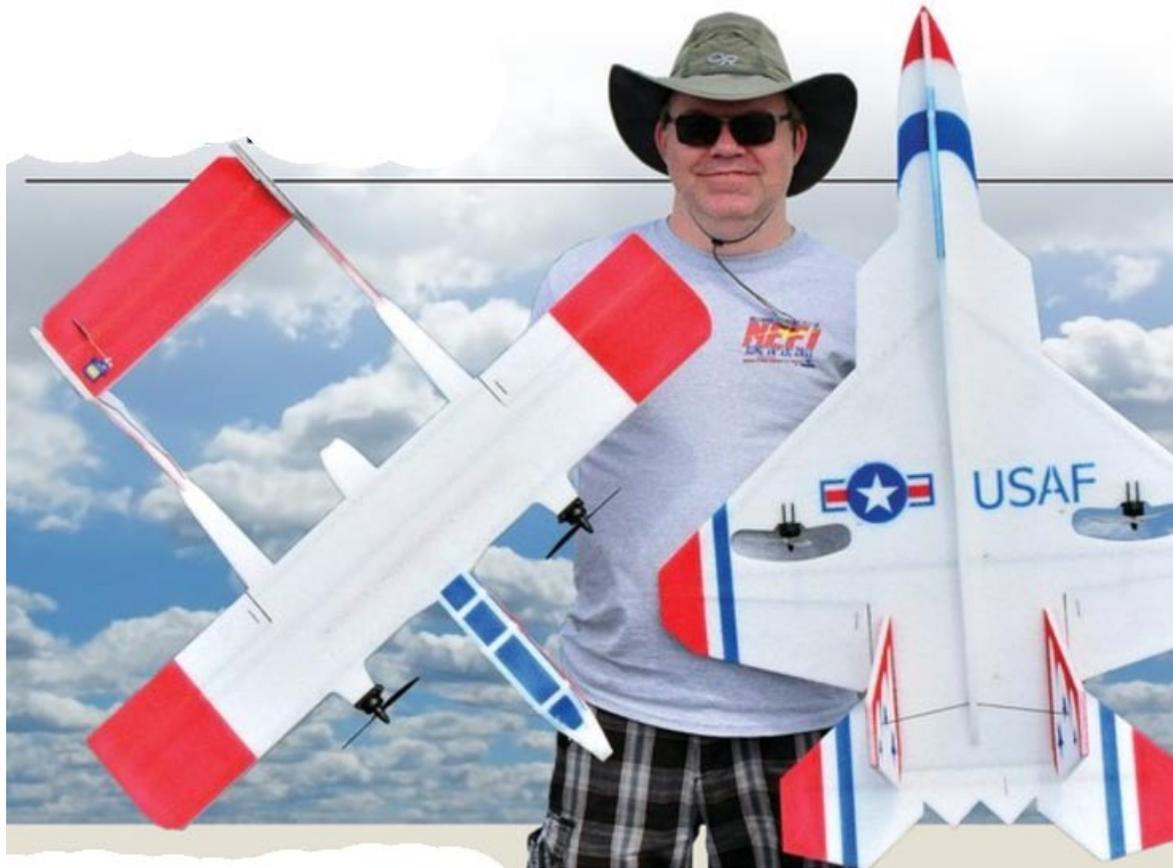
Neat looking arrangement of two motors in the F-22. Thrust right in front of the ailerons. Of course differential thrust would provide some interesting aerobatics too.
