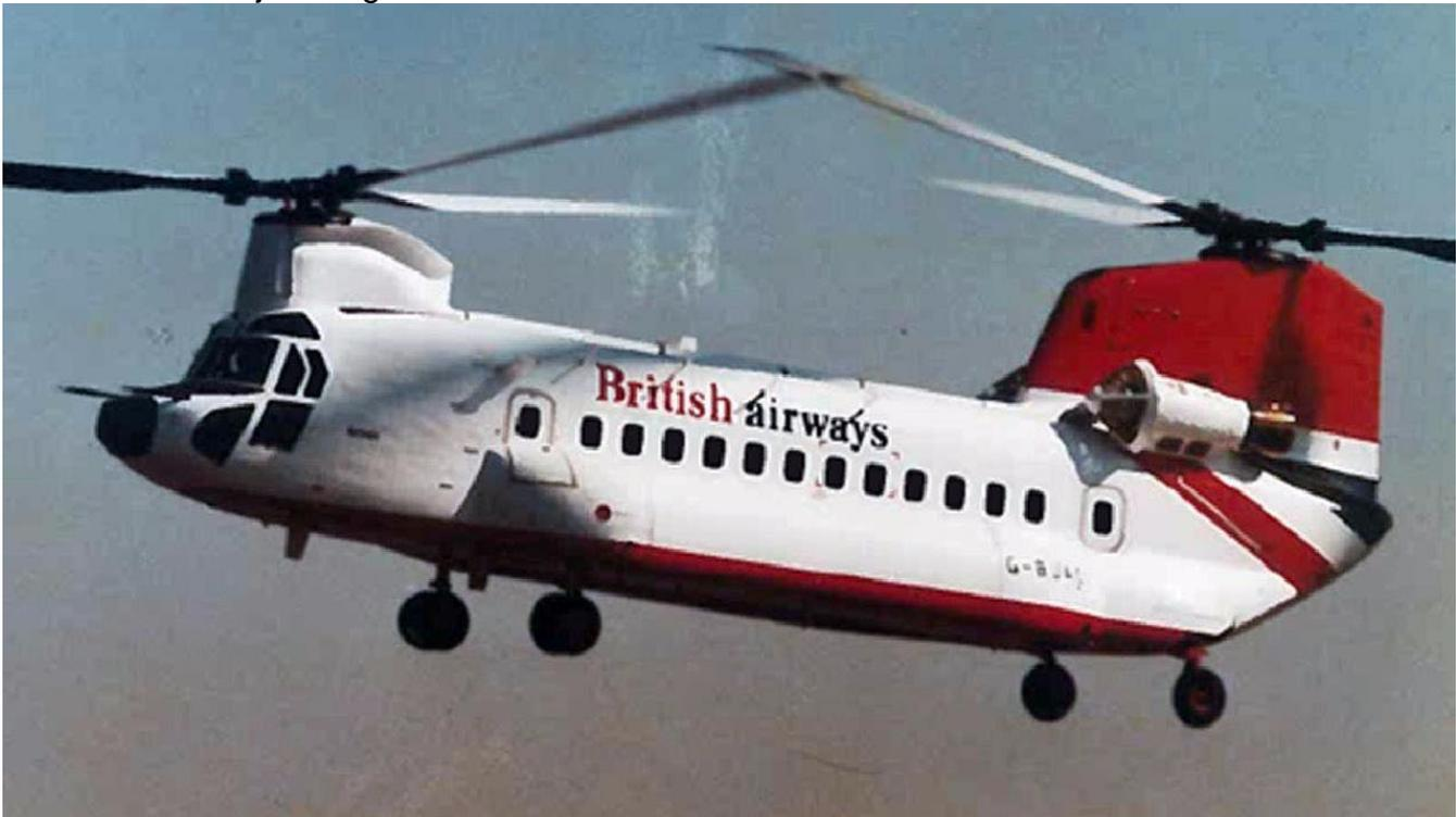
First new thing was the need for larger fuel tanks to allow longer missions and avoid refueling on Oil Rigs where possible. Second thing, enhanced by the bigger tanks, was the requirement to ditch and live in water with high wave states.
