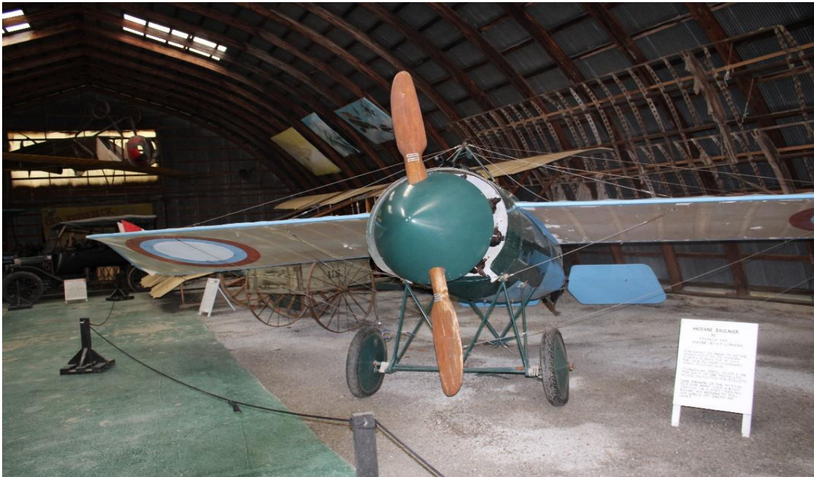
Figure 7 Marane Saulnier N French 1914, 80 Hp Lerhone. Grand-Daddy of Modern Fighters.. First to carry a forward firing machine gun. Steel plates installed on the back of the props to deflect bullets
