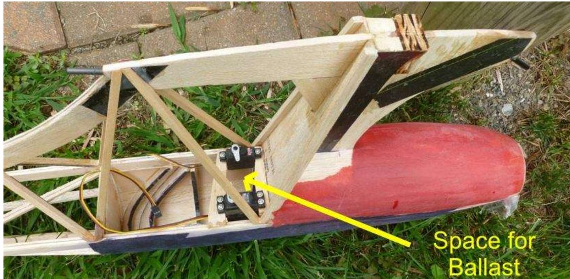
Now the challenge was to make a piece of ballast that fit this space and weighed 15 oz. This could only be satisfied with a molded lead piece. So I set about making a mold from some pieces of wood into which I would melt old lead tire weights. Fortunately my son works for Subaru and we regularly harvest the crop of castoffs.
