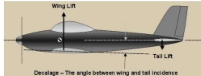
The chord line is an imaginary line through the airfoil running from the furthest forward point on the leading edge to the furthest aft point on the trailing edge. If we find the chord line of the wing and the chord line of the horizontal tail, the angle between them is the decalage.
