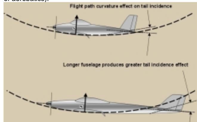
Having a short tail moment arm will help the turn rate, or the radius of the "turn" about the pitch axis, but it also makes some of the other factors, especially the effect of the wing's aerodynamic pitching moment coefficient, more critical.
