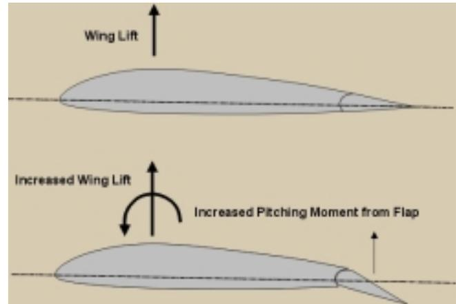
Conversely, a well-forward hinge line location will tend to minimize the effects on the aerodynamic pitching moment coefficient, and maximize the other two effects. On some of the models Joe and I experimented with, we used hinge line locations around 20% of the chord back from the LEADING EDGE of the wing. Aerodynamically this can have all sorts of interesting and mostly beneficial effects, but structurally it can be an engineer's worst nightmare!
