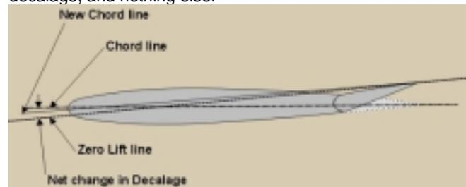
If you have a conventional elevator + stabilizer ("two element") tail, then you also altered the camber of the tail's airfoil, which changes its zero lift line, in addition to changing its incidence. The change in the zero lift line is in a direction
