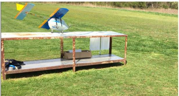
It apparently failed as the torque from this propulsion system overwhelmed the landing gear resulting in a powered roll off the table.
