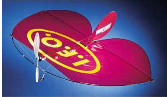
Dan Kreigh's IFO ( Indoor Flying Object ) is an example of an indoor aerobatic R/C plane with light loading. The IFO is 33-inch wing span, weighs about 7 oz and is powered by a Speed 280 with a gearbox. From our formulas it should fly at around 13 feet/sec. It is quite agile and has been impressive in indoor sites.
