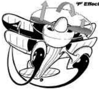
**The P Factor causes the prop to produce a yawing moment in high angle of attack flight**
