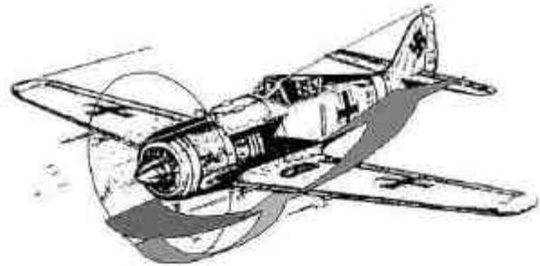
**The swirling prop wash effects can induce rolling and yawing from interference with the airframe**
