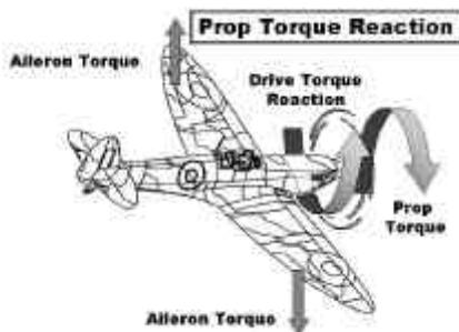
**Propeller torque can usually be counteracted by aileron deflection.**
