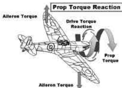
**Propeller torque can usually be counteracted by aileron deflection.**
