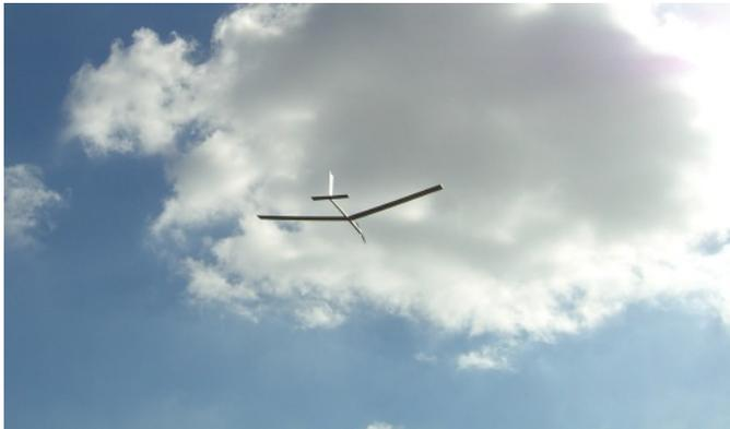
It floated out of my hands into the modest breeze but control was initially a handful as the fuselage was very soft in torsion. When Dale put rudder control input the fuselage would twist and take out much of the control force. It took a little while for him to sort it out following which it floated around with practically no power input. Watch this space to follow his progress.
