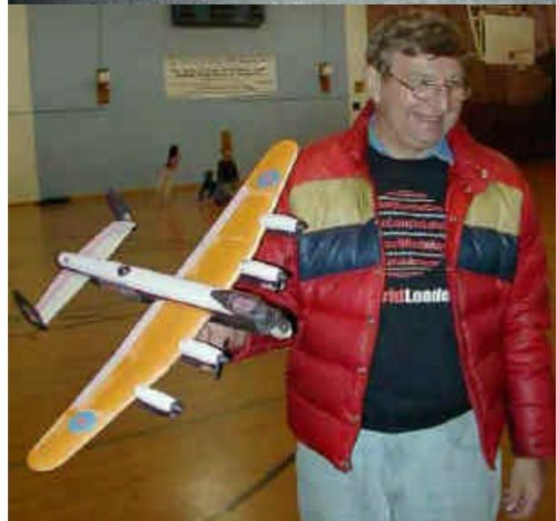
Did it fly? Not quite, at 77 grams with the detail added it made another long gently turning descent then broke a prop and I didn't have a spare with me. But the wizard, Doc, tells me that I still have the wrong props and it should fly. If not I can add the other two motors. Although it may not be suitable for indoors at that weight I could also add an Rx, and ESC and two servos for another 30grams then I'll have a Jim Dandy four motor outdoor flyer!
