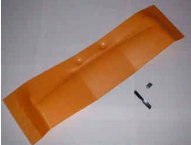
There was a molded foam-sheet 17-inch wing with a flat center section and dihedral tip sections, a minute N20 motor and 3 inch prop. "Should be able to build a model light enough to fly with two 50 mah NiCad cells". "There are a variety of Nocal profile scale designs on the web, why not make a Hurricane?"
