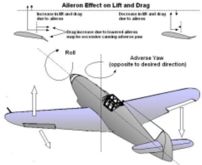
If the plane has lots of dihedral and the ailerons are only of average efficiency, the adverse yaw could couple with the dihedral to cancel out much, if not all, of the ailerons' rolling effect. However, very efficient ailerons can avoid this problem. It can be done, but the typical proportions used for ailerons usually can't do it.
