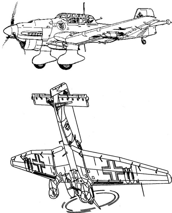
If we ignore the stub sections next to the fuselage, the Ju-87 Stuka has about 9 degrees of dihedral per side, measured at the chord line of the airfoil. The stub sections
