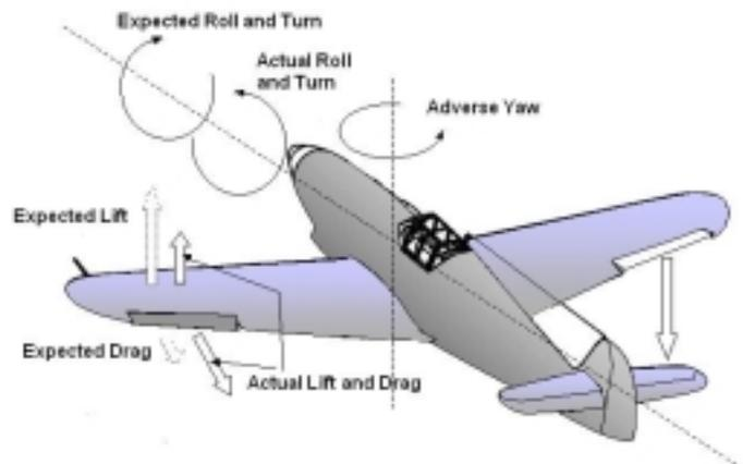
Spin recovery on an airplane with no rudder can be a problem as well for the same reason. In addition, if the ailerons are used as flaps, the combination of downward flap deflection plus aileron inputs can act like reverse differential, making the adverse yaw problem extremely severe.
