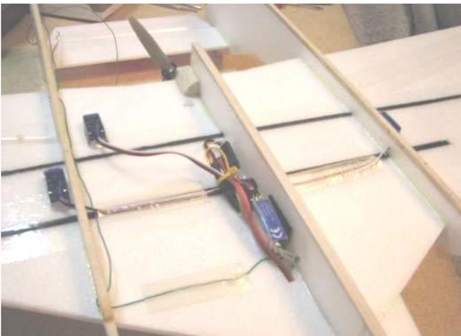
The motor installation on this version uses an outrunner motor mounted on a GWS 10 mm gearbox stick mount. Note the 10 mm stick bonded to the foam fuselage.
