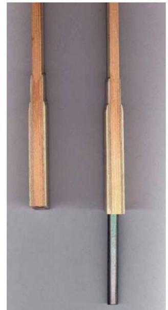
I use carbon rod for the wing joiners. I think I could have used 1/4" rod but preferred 3/8" to be on the safe side. For the main spar I used #R-24, 3/8" solid carbon rod. The secondary spar used #R-10A, 5/32" solid carbon rod, both supplied by: Aerospace Composite Products,; Info@acp-composites.com Website: <http://www.acp-composites.com/>
