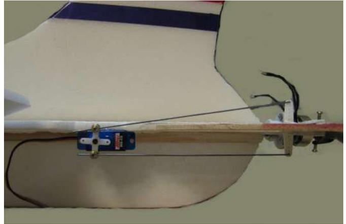
She obviously understood the finer points of making such a system work as she made the control horns parallel and equi-distant from the pivot. This control geometry is perfect over the whole range of motion, and obviously quite rigid; also it works!
