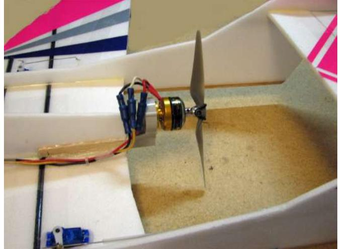
Chellie's other foam jet was a simple delta with a tractor motor. The inspiration came from a 20 x 30 inch sheet of foam board
