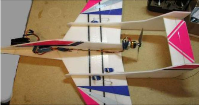
Here again the sophistication is not obvious, but the simple installation of the servos provide short stiff connections to the ailerons and the two graphite rods provide both bending and torsional stiffness to the simple wing.
