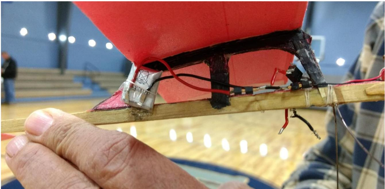
Besides Lipo or Nicad/NiMh batteries there is another choice for us electric motorheads i.e. the high capacity capacitor. My black/white flier uses two capacitors to supply power.
