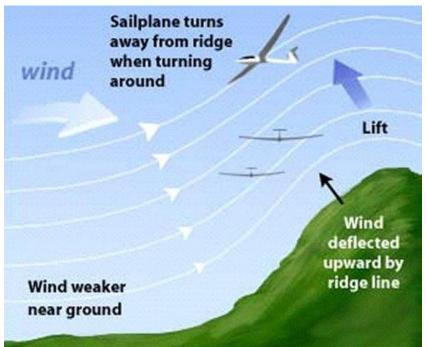
When you fly a model into this updraft the lift, and the lift velocity is greater than your model sink speed, staying in the lift zone constantly turning and flying back and forth parralell to the slope, you can stay aloft as long as you and the wind hold up.
