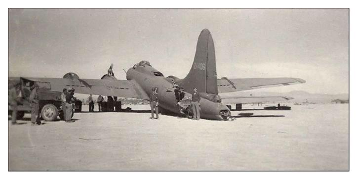
Although the tail actually bounced and swayed in the wind and twisted when the plane turned. All of the control cables were severed, except one single elevator cable still worked, and the aircraft miraculously still flew!
