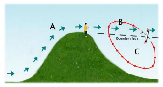
The dynamic soaring pilot will let the aircraft fly downwind in the high velocity zone B, where it picks up speed, and then dives into the calm zone C turned around and back up into the high velocity zone. This cycle is then repeated over and over. With the right conditions and good piloting, each time the aircraft completes a cycle it will pick up more speed.
