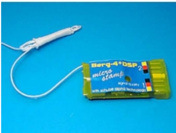
It weighs only seven grams, about 1/4 ounce but has all the high tech signal processing and features an indicator lamp, which indicates the number of glitches filtered out during the last flight.
