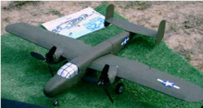
His second airplane was a B-25 at about 30 inches span. This airplane has a fixed gear but had no problem with the rough surface. In fact the flight performance was sparkling. The airplane was powered by two Light Stick motor / gearbox assemblies (less than \$20 each) it had a built up balsa / tissue wing. The fuselage and nacelles. were carved from foam, covered with tissue and painted.
