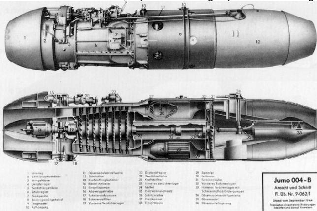
**Junkers Jumo 004 axial flow engine**
