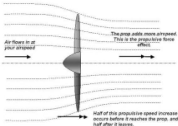
If the air has to be accelerated in order to make thrust, then the speed of the air in the slipstream behind the prop MUST be faster than the airspeed of the rest of the airplane. This speed difference is what we loosely refer to as "slippage".
