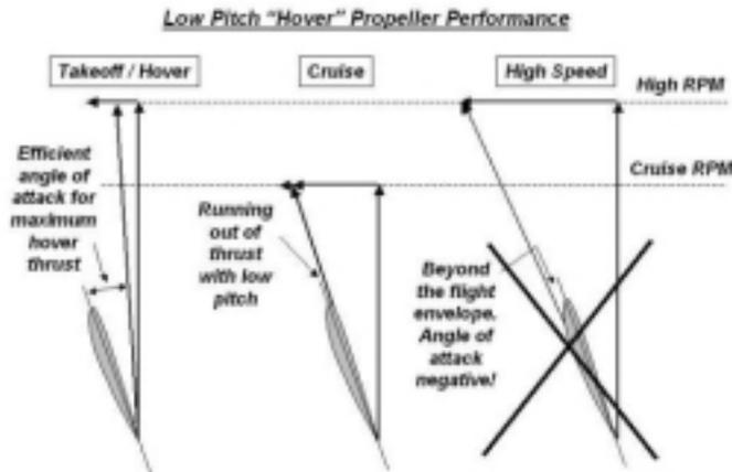
If we select our propeller to match the high-speed flight performance we may not be able to take off due to the propeller operation in deep stall, although the cruise condition may be efficient.
