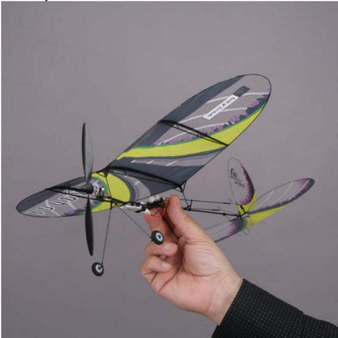
At only 15 grams, about half an ounce, including three channel 2.4 GHz RC unit this is a marvel. And, as I mentioned in the prior discussion of Parkzone's outdoor models, all their new 2.4GHz radio systems are compatible with the Spektrum radios.
