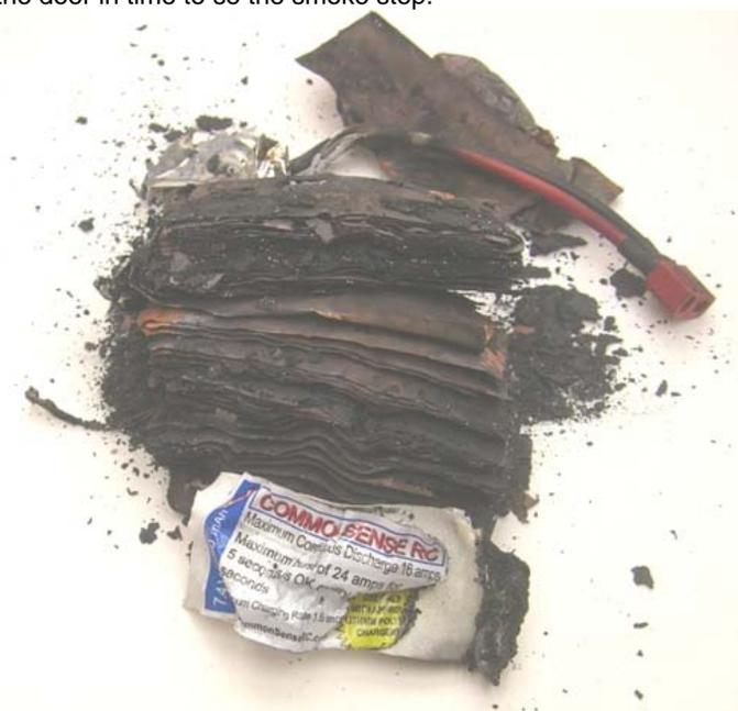
The reason for the flare up; Not definite but a theory; I was charging a two cell LiPo that showed about 7.9 volts, and I wanted to top it off. I think it is possible that the automatic cell count read the battery as a low voltage three cell, overcharged and toast. (Not unusual problem with the early automatic LiPo chargers causing quite a few re-calls Ed.)
