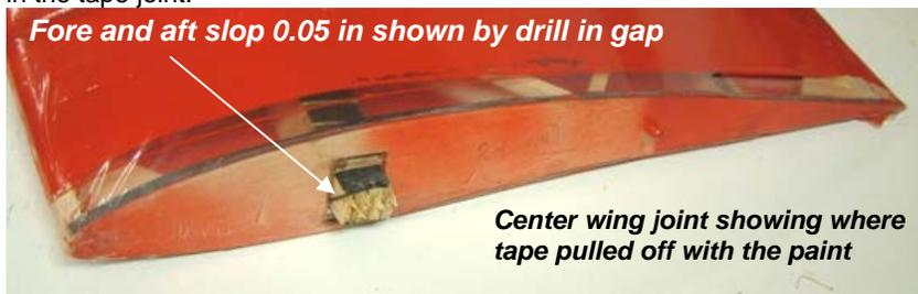
Fore and aft slop 0.05 in shown by drill in gap
