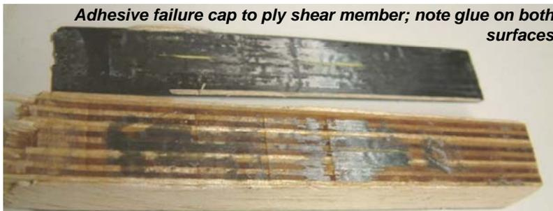
Adhesive failure cap to ply shear member; note glue on both surfaces
