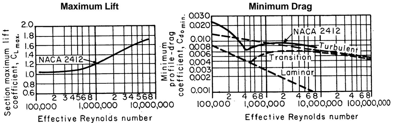
Scale effects on the maximum lift and minimum profile drag on the NACA 2412 airfoil
