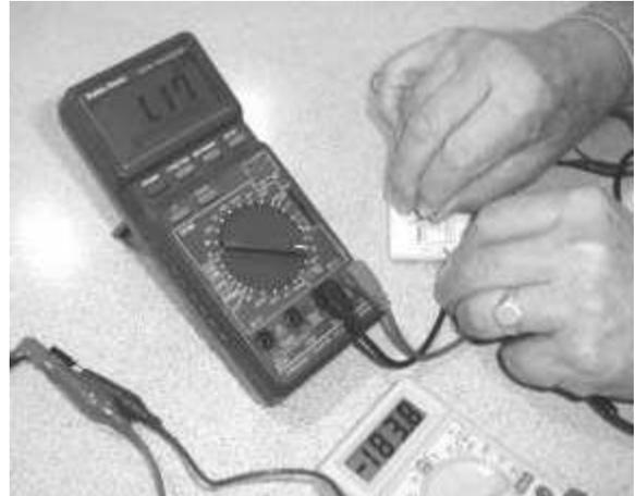
The picture following shows the setup to load test the pack. The hair dryer is the load and at 4.56 volts it is producing 191 milliamps. Once you measure the load-current it is not necessary to measure both voltage and current simultaneously. Just measure voltage during discharge so you know when it's done.
