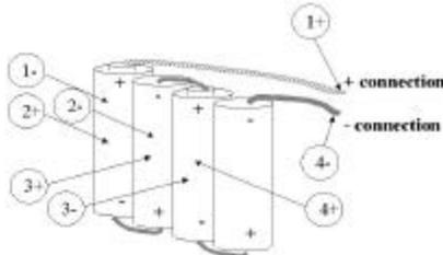
Do this with a pin or needle clamped in an alligator clip test lead and connected to our DVM. You need two pins and test leads so you can connect to both positive and negative probes. Just insert the probes, at the noted pairs of points, for measurement of cell 1, cell 2 etc.
