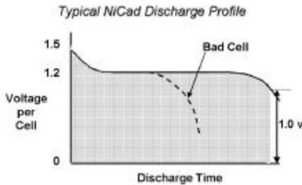
Customary end of timing is when the pack is down to 1 volts per cell. In the case of the Rx battery that would be 4 volts.
