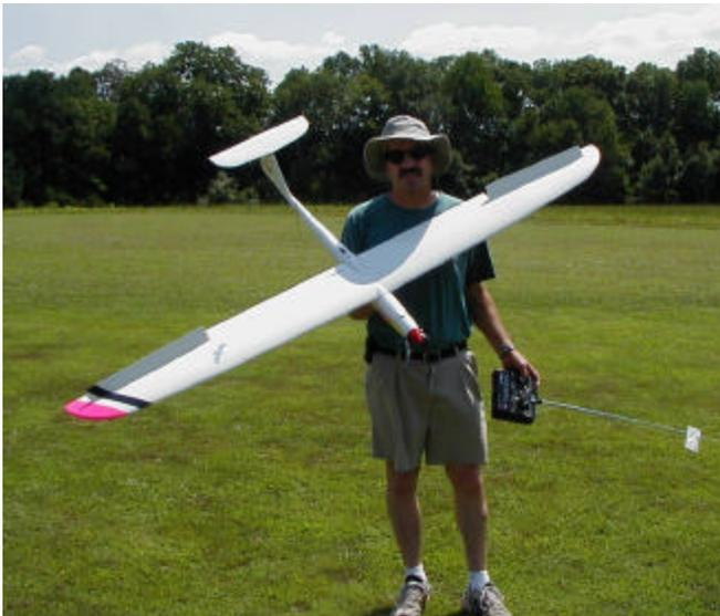
An exciting plane to watch was Ed Berchtold's Surprise. With a current draw of 80 amps, the plane accelerated upward for only four seconds before leveling out at a high altitude. The F5B class airplane is designed for fast climb, soaring, and spot landing. It uses an Aveox F27L motor with a 15x13 prop and 25 batteries 1250 SCR.
