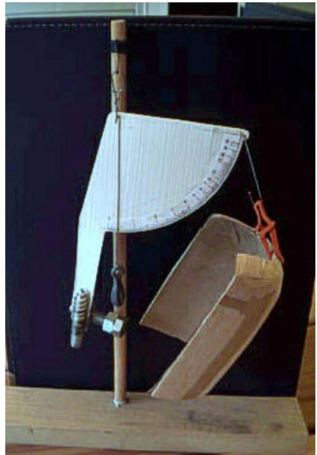
The scales are surprisingly accurate and durable. They don't work with a spring that can loosen with time. They basically compare the weight of your object to the scale itself and once calibrated work for a long time. The bulk of the scale is constructed from wood or plastic. Mine were made from heavy plastic leftover from the siding of my house. Light plywood would work just as well.
