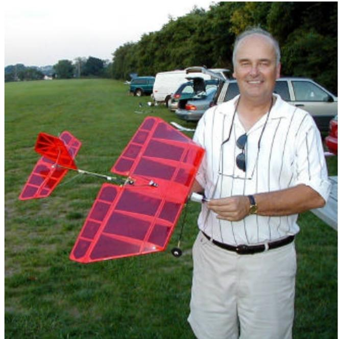
Bill Groft performed aerobatic flights with his 1.25X Fast Freddie plane, from Anything-RC. The plane, able to fly vertical, uses a Hacker B2-15L brushless motor with a 4:1 gearbox, APC 10x4.7 prop, Jeti 18A speed controller, and 8 KR600AE batteries.
