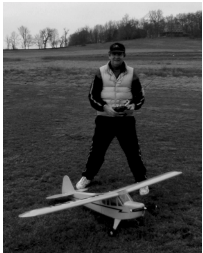
Newsletter Editor, Dave Harding with his Hanger 9 Piper Cub. Electric powered by an Aveox 1409/2Y and 24 x 1700 mAh NiCad cells. It's overpowered!
