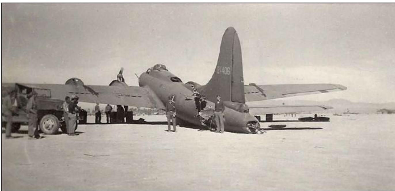
Although the tail actually bounced and swayed in the wind and twisted when the plane turned. All of the control cables were severed, except one single elevator cable still worked, and the aircraft miraculously still flew!
